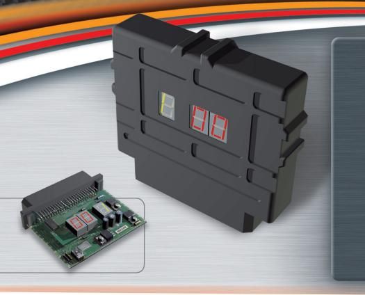
The Active Differential (ACD) is extremely important for vehicle traction. The ACD computer was designed based on data collected from the production cars of the World Rally Championship. It enhances and facilitates the work of the whole team during races and complies with FIA regulations.
